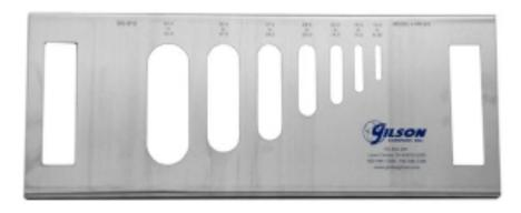
Grid sieves (for flakiness test)
