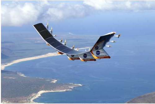
NASA Dryden Flight Research Center Photo Collection http://www.dfrc.nasa.gov/gallery/photo/index.html NASA Photo: ED01-0209-6 Date: July 14, 2001 Photo by Nick Galante/PMRF The Helios Prototype flying wing is shown near the Hawaiian islands of Nihoa and Lehua during its first test flight on solar power from the U.S. Navy's Pacific Missile Range Facility.
